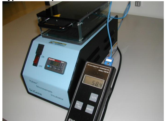
Digital Thermometer connected to Micro Incubator. Temperature agreement is 0.1 °C
